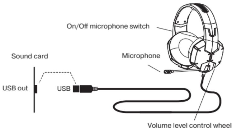
Fig. 1. Connection diagram
